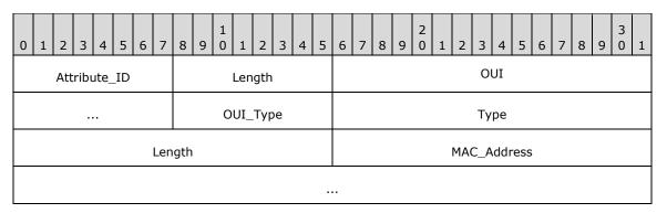
**Attribute\_ID (1 byte):** Contains the ID of the element as specified [IEEE802.11-2007] section 7.3.2. It MUST contain a value of 221 (0xDD), identifying a vendor-specific element (as specified in [IEEE802.11-2007] table 26) in which the vendor is identified by an IEEE-issued OUI.
